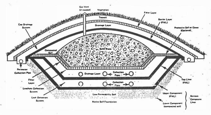
WHAT IS A LANDFILL? A secure landfill is a carefully-engineered depression in the ground (or built on top of the ground, resembling a football stadium) into which wastes are put. The aim is to avoid any hydraulic [water-related] connection between the wastes and the surrounding environment, particularly groundwater. Basically, a landfill is a bathtub in the ground; a double-lined landfill is one bathtub inside another. Bathtubs leak two ways: out the bottom or over the top.
